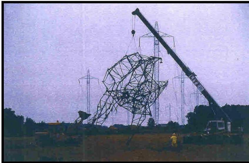
Figure 2.5 - dc Tower Failure under Microburst (High Intensity Wind)
