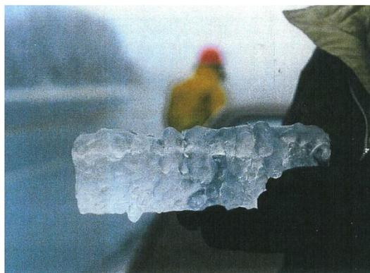
Figure 2.2 - Glaze Ice Sample from Conductor (1984 Storm)
